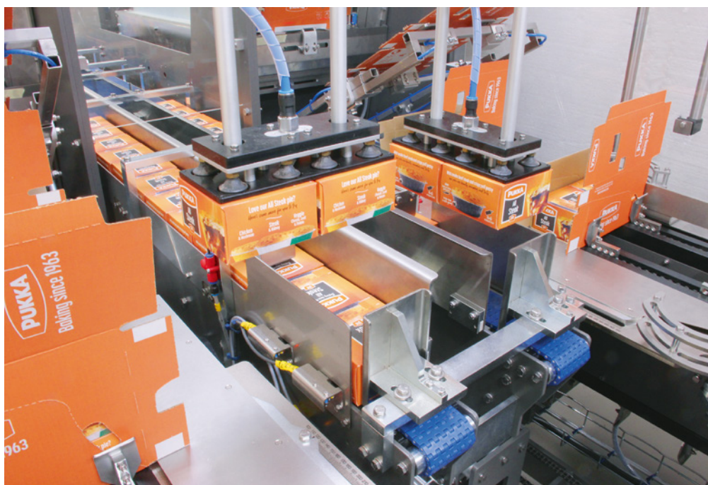
Dual 'back to back' pick and place robots
